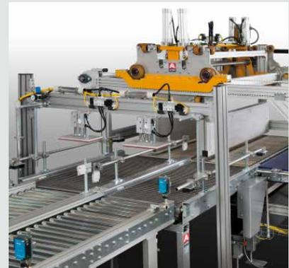
» 2-, 3- or 4-axis modular robot system in portal frame design for palletizing.
