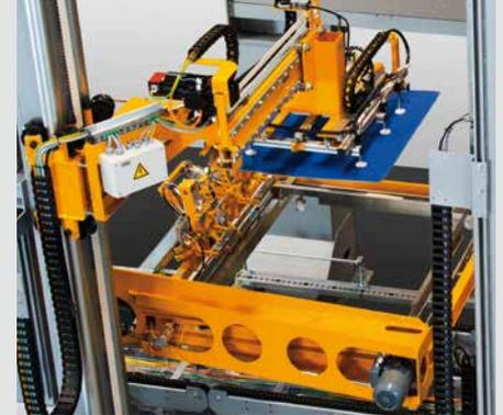
» The sweep-off depalletizer transfers layers of various configurations of round, oval, rectangular bottles, PET and HDPE plastic containers or cans onto a discharge table and leads them into the filling process.
