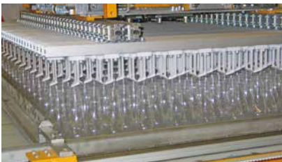
Without pressure, bottles are combined to a complete layer on a tray. The bottles are held safely from all sides during this process.
