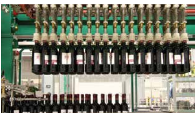
Multi gripper heads with automatic adjustment, diameters from 56 to 110 mm. Packing of round, oval and square bottles.
