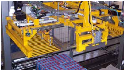
CP-Palletizing system with 3 or 4 axes for cartons, trays and shrink packs. Palletizing of complete layers or row by row.
