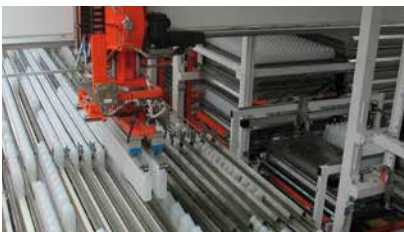
Empty plastic bottles are taken from the conveying line sort by sort with a 2 axes tray loader and placed on a provided tray then placed back on the selected line.
