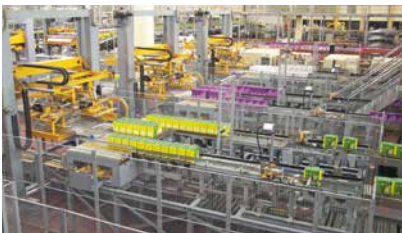
2-axis high performance palletizer for palletizing of beverage cartons. Each palletizer has two high-speed infeeds. Formation of layers is effected in an almost touch-free way.
