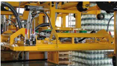
Bulk glass take-off depalletizer, grips layer by layer by means of vacuum plate. Interlayer and empty pallet handling are integrated.
