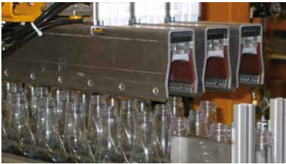
Empty PET bottles are palletized with AUTEFA Solutions row gripper system.
