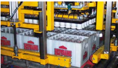
Palletizing and depalletizing system for crates with integrated glass bottle handling system.
