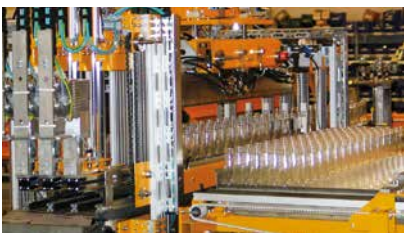
Fully automatic palletizing system for plastic containers. Handling of empty pallets, interlayer and top frames.
