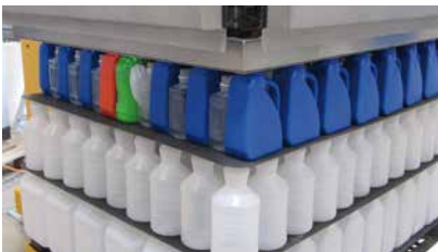
Universal gripper head for a gentle handling of plastic containers. Palletizing & Depalletizing of complete layer with AUTEFA Solutions Vacugrip.
