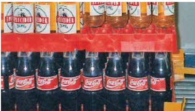
Palletizing of bottles in plastic display trays. The bottles are gripped by means of single grippers or row grippers.
