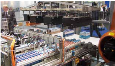
Fully automatic sorting installation for beverage cartons for arrangements of 2x6, 2x8 and 3x9 by means of exchangeable gripper heads.
