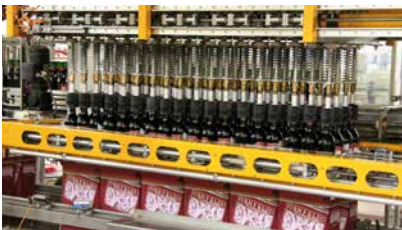
Set packer for packing bottles into cartons. The multi gripper head which can be adjusted on 4 axes automatically, combined with centering frame adjustable on 3 axes avoids cost-intensive changing of format sets.
