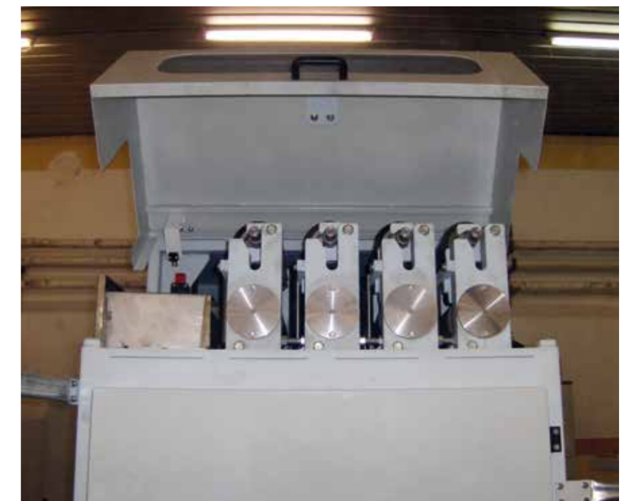
Sliver Drafter with four couples of cylinders
